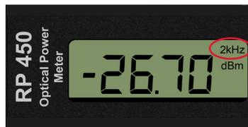
The 2kHz tone output of the DLS 350 will be recognized by ODM power meters to provide a fast, simple continuity test on MM fiber.
