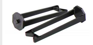
These black plastic rings flex at the end for easy insertion or removal of cross connect cables. The 3/8" 1/4 turn connecter mounts on the front and back of the Mighty Mo racks. It can also be installed into 3/8" square accessory holes on the sides of the Mighty Mo racks or into any open 3/8" square EIA mounting hole.
