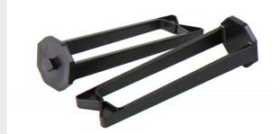
These black plastic rings flex at the end for easy insertion or removal of cross connect cables. The 3/8" 1/4 turn connecter mounts on the front and back of the Mighty Mo racks. It can also be installed into 3/8" square accessory holes on the sides of the Mighty Mo racks or into any open 3/8" square EIA mounting hole.
