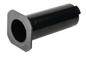
Cable management spools effectively manage excess fiber cable slack, providing flexibility and the proper bend radius for cables. They mount at rack unit intervals on the front of the 6" wide vertical manager or on the front and rear of the 10" and wider vertical managers with fingers.
